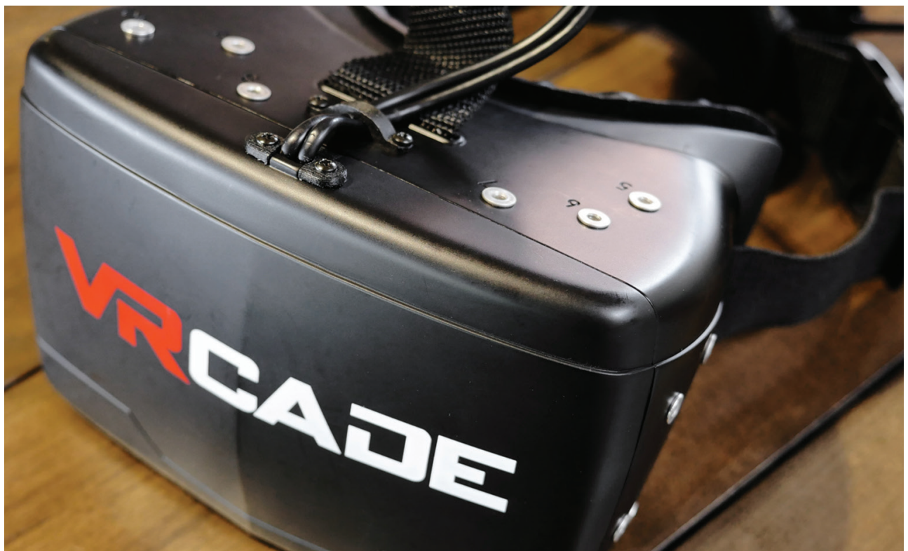
VR Studios simplified their production of virtual reality headsets by opting to 3D print parts instead of tooling-up. What would have been a four-part enclosure was consolidated as a two-part assembly in FDM.
